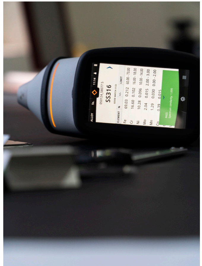
Photo of Scanjet Spectrometer and material passing the SS316 requirement. Photo: Gabriel Brännlund
