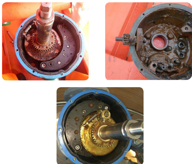
Drive units for tank cleaning machines in three different conditions. Water ingressed, corroded and normal condition.
