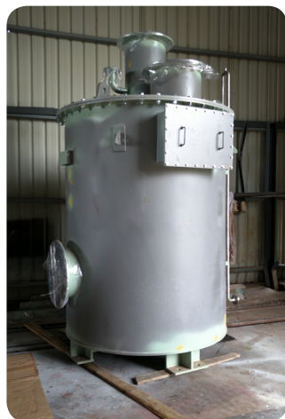
Deck Water Seal ready for painting
