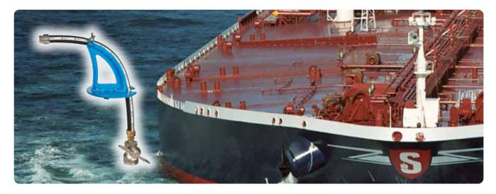
Turnaround time is crucial and the tank cleaning period should be kept to a minimum, In most cases this is achieved by fixed equipment but Scanjet can also provide portable tank cleaning machines to reduce time and cover any shadow areas in the tanks. The portable machines are normally twin nozzle, turbine driven and
