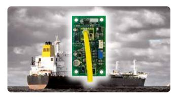
The SML-1000 electro pneumatic system offers continuous measurement providing DC 4-20 mA or digital Modbus outputs to central display units, to Integrated Alarm Monitoring System and to Loading Computer. The largest systems delivered is composed of 20 cabinets in different fire zones, which monitor more than 250 measuring points.
