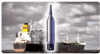
Custom-made high-quality pressure transmitters measure absolute or gauge pressure depending upon the application. Transmitter construction is fully laser welded and internally encapsulated to ensure complete sealing. Materials of construction are SS316L, Titanium, Hastelloy to suit all shipboard fluid. All are rated IP68 and suitable for permanent submersed operation. Transmitters are Marine Type approved and Certified Intrinsically Safe for hazardous Area applications.
